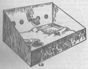
Commercial type of vivarium heated by electric light bulb. Glass over top. Perforated zinc over ventilation holes. For lizards or snakes.
